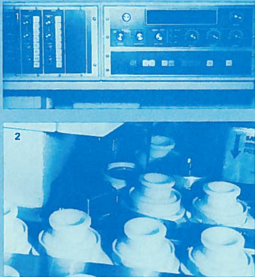
1. Control panel for the gamma counter. 2. Sample changer of the gamma counter.
